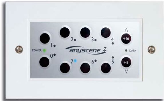
23 scene 256 channel DMX scene recall unit. NEW FEATURE - Now multiple units may be used in one DMX installation.
